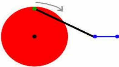
A rod is connected to a rotational crank, by moving the rod a circular motion is created. Alternatively, turning the rotational crank creates a linear motion.
